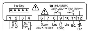
NOTE: In model with 110Vac the power supply has to be connected to 6-7 terminals
