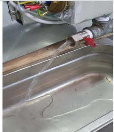
STEP 5 : Open the Boiler tap and fill the boiler with Limescale cleaning solution or vinegar ( 300ml ) **Attention: Do not drop liquids to the electrical parts !!!**
